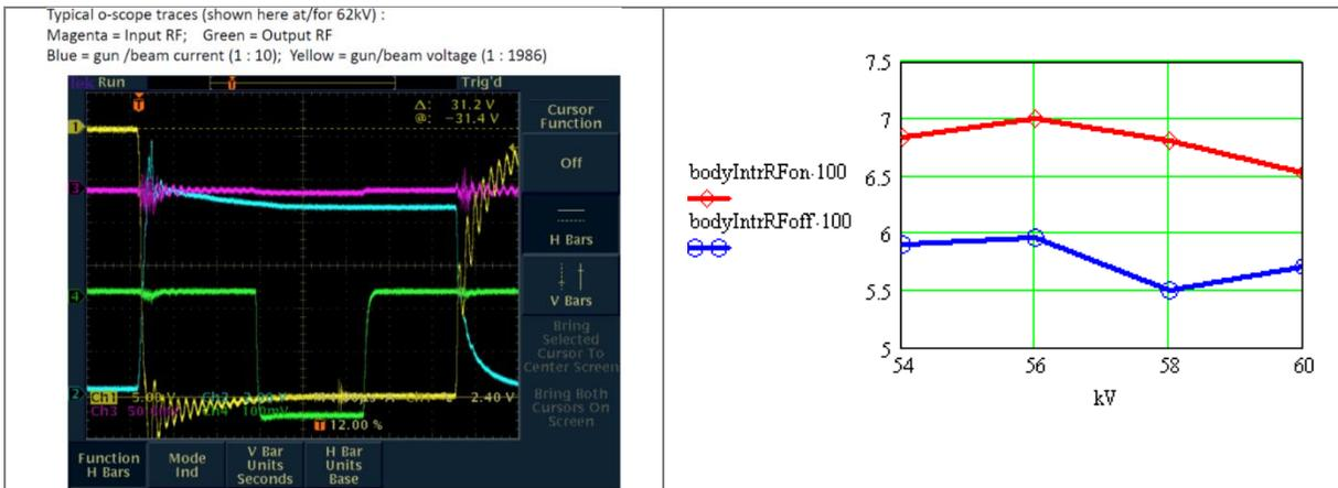
**Figure 2. (Left)** Traces of gun voltage (yellow); beam current (blue), output power (green), and input power (magenta); the horizontal scale is 5 micro-secs per div. **(Right):** Inferred body intercept measured as a percentage of beam-power with RF on (red) and off (blue)
