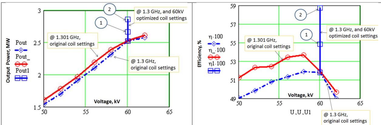
**Figure 3. (Left)** output power (MW) vs beam voltage (kV) at 1.300 GHz and 1.301 GHz, as measured via calorimetry on the matched load. **(Right)** Efficiency as a percentage of beam-power. The currents in matching and focusing coils were optimized to obtain higher output powers as shown by points 1 and 2
