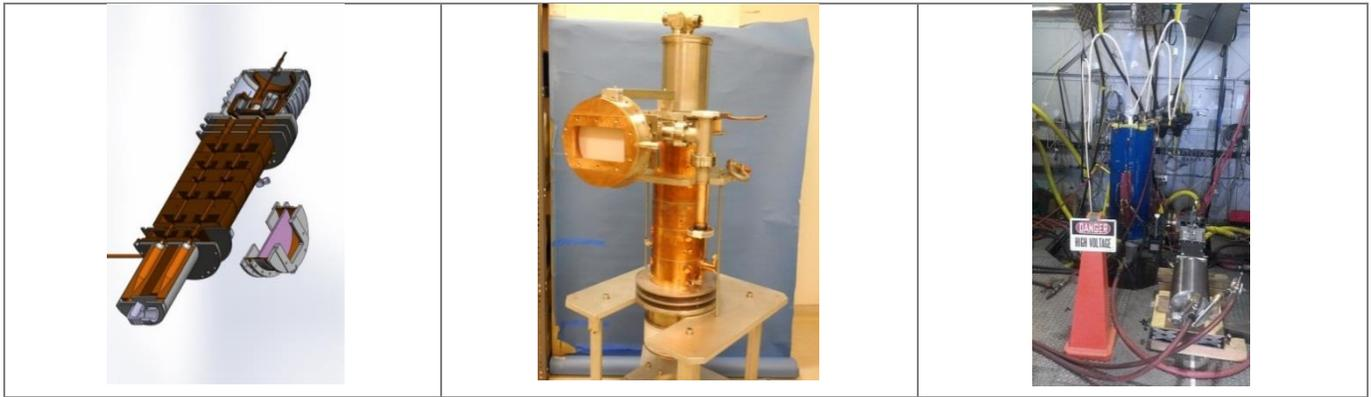
**Figure1. (Left)** a 3-D cut-away view of the tube; **(center)** photo showing the tube before it was inserted the magnet assembly; and **(right)** the test-setup, showing the klystron (in blue magnet), RF-window, and RF-load, during installation at the CPI test site
