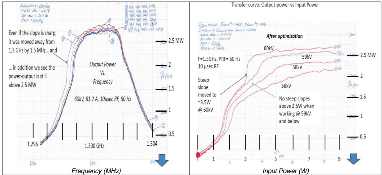
**Figure 4 (left)** example of investigations of the bell-jar shape of the dependence of the Output-power vs. the RF frequency at 60kV vs. different coil settings. **Figure 5 (right)** An example of a family of transfer curves for the coil settings that minimized the body-interception. [ Input power is in Watts (horizontal axis)]. The coils are set to "Optimized 1" (see Fig.3)
